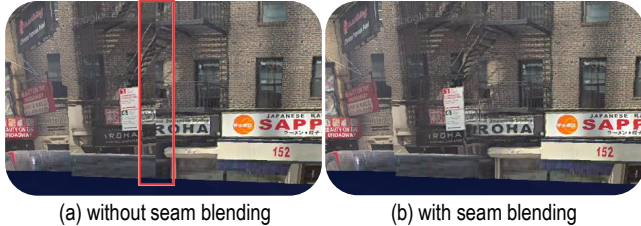
Figure 4: Results before and after applying the weighted alpha blending near the seams. (a) Without blending, the seam (highlighted in the center of the red box) at the edges is noticeable due to the texturing misalignment. (b) Weighted alpha blending in the fragment shader makes the seam much less distinguishable.
