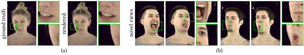
Fig. 8. Limitations. While our method achieves good image quality in general, it suffers from some drawbacks. (a) Since we export only view-independent radiance to the texture, we cannot render specularities such as the ones on the nose, teeth and cheeks. (b) At extreme out-of-training-distribution viewpoints, our method sometimes exhibits shell artifacts due to transparency of the layered mesh from grazing views. Please refer to the supplementary material for video visualizations.
