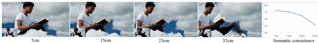
Figure 6: Result with different stereo baselines. Unnatural artifacts begin to appear as the baseline expands. Our method performs well for stereoscopic video generation where baseline is usually less than 7cm.
