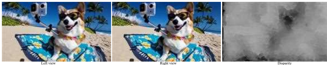
Figure 14: Results of Deep3D. Deep3D does not provide the function to change the stereo baseline, and the vague disparity map on the right side demonstrates its weak stereo effects.
